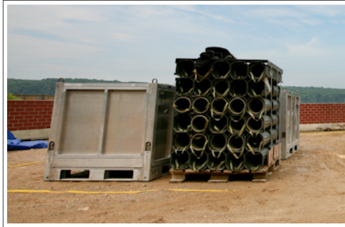
Figure 1-4: These are two kinds of pallets: on the left is an empty JMIC (Joint Modular Intermodal Container), and on the right is a wooden pallet loaded with inert ammunition.
